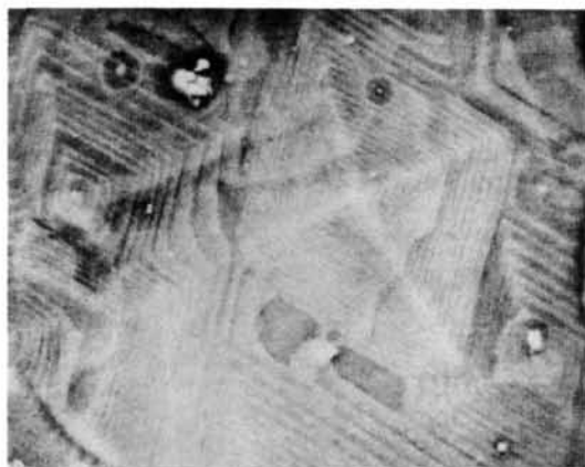
Fig. 1. Elementary monomolecular spiral on crystal of the monoclinic form of tetratriacontane ( C_{34}H_{70} ) (900 \times ).
